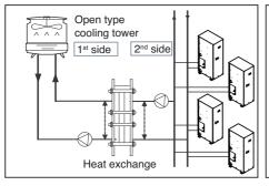
[Open type cooling tower + Second heat exchanger] Heat exchanger is installed between the cooling tower and outside unit system piping, and the temperature difference between 1<sup>st</sup> side and 2<sup>nd</sup> side is maintained constantly
