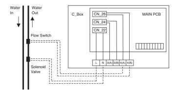
Set the DIP switch refer to Fig.1 and turn on the power when you individual control for water solenoid valve control.
