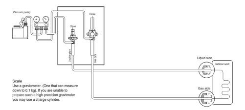
Note : Always add an appropriate amount of refrigerant. (For the refrigerant additional charge) Too much or too little refrigerant will cause trouble. To use the Vacuum Mode
