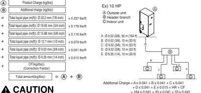
If a negative result is obtained from the calculation, no refrigerant needs to be added.
