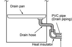
\*Connect and fix drain pipe at outside of the unit on site.
