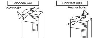
A hole on the wall fixing bracket for the indoor unit is a long hole. Therefore the indoor unit can be fixed at any position keeping clearance from 0 to 50 mm.
