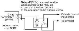
Note) Determine the cable length between the indoor control P.C. board and the relay within 2m.
