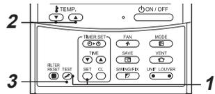
**1** When pushing SET and TEST buttons for 4 seconds or more, following display appears.
