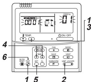
**1 Push and hold  $\text{TEST}$  button and “TEMP.” button simultaneously for at least 4 seconds. After a while, the display flashes as shown in the figure. Confirm that the CODE No. is [01].**
